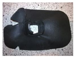
The original rubber flexible boot that fit around the clutch lever became hard and cracked over time.
