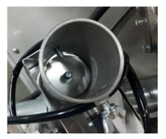
View of flapper inside of the controller where resin would escape the system.
