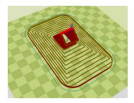
INFILL: 60% LAYER THICKNESS: 3 perimeters
