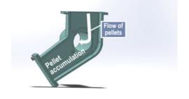
Cross-section of the area where extrusion pellets accumulate and were unable to transfer to the extruder.
