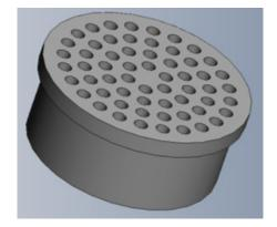
INFILL: 100% RETRACTION: none PRINT TEMP: 235°C PRINT TIME: 1 hour
