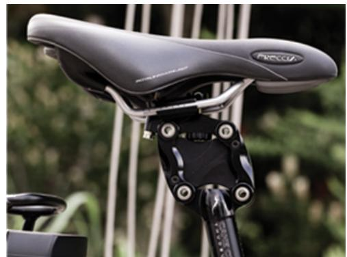
The original Thudbuster LT seat post uses 2 urethane cylinders stacked on top of each other inside of a hinged parallelogram to provide suspension through the round tube.
