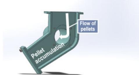
Cross-section of the area where extrusion pellets accumulate and were unable to transfer to the extruder.
