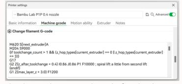
The Change Filament G-code can be found in the **Machine Gcode** tab of the Printer settings window.
