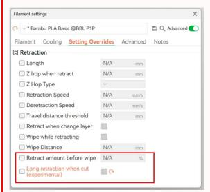
A long retraction can pull softened filament into the cutter, causing it to deform instead of being cleanly cut. This can lead to the filament getting stuck and potentially causing an AMS failure.
