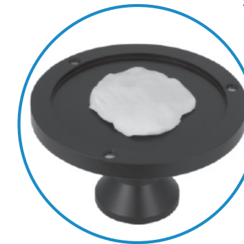
Support with plasticine for adaptable positioning
