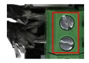
Pull the Heating Rod cables out from the Mounting Block from the bottom.
