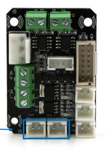
Insert the cables of the Heating Rod into the terminal and tighten the screws to fix. Ensure there is no exposed wired touching with each other, or it may do harm to the printer.
