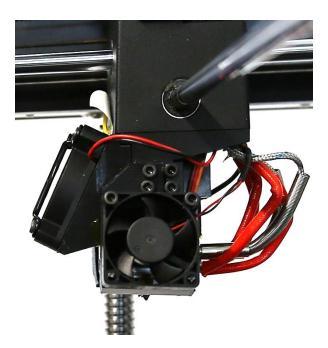
Grab the connector of the new Fan by tweezers out from the top to help it go through the Mounting Block.
