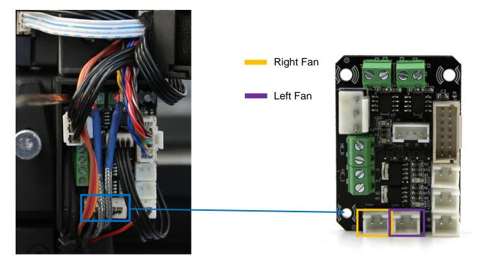
• Cut the old cable off. Take the old Cooling Fan and the its cable out.
