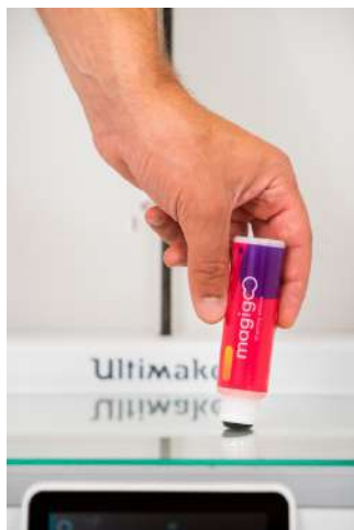
Figure 15: Apply Magigoo in an even layer on the area for printing, for a more detailed application guide visit (insert link to videos)
