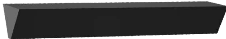
Figure 8: Wedge print, an ideal geometry for testing the first layer adhesion of your build surface, the narrow base limits the contact area with the build plate. This shape is one of the geometries used in the Magigoo testing labs to assess the adhesive performance with different material and adhesive combinations.
