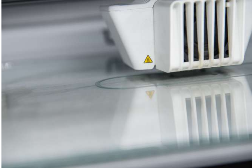
Figure 18: Tweaking the first layer extrusion settings can help with improving first layer adhesion
