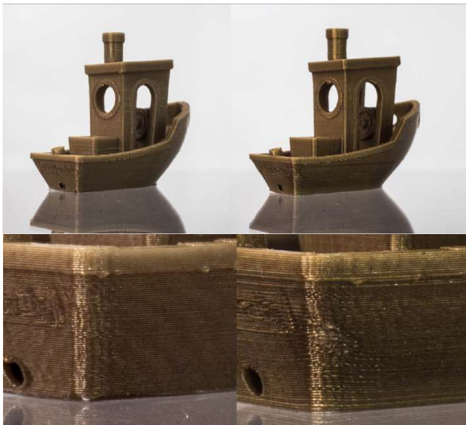
Figure 6: Benchy print using PLA, images on the left shows a benchy printed with the heated bed set to 60 °C, while the images on the right show a benchy printed at 80 °C, on closer it can be noted that the benchy on the right warped and also shows artefacts due to the layers curling up from excessive heat.
