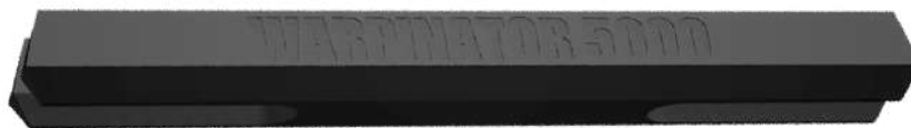
Figure 9: The Warpinator 5000 by Maker's Muse, this is a similar concept to the wedge print but slightly more extreme.
