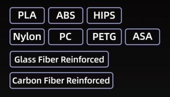
Note: Glass fiber reinforced and carbon fiber reinforced filaments need to be used with a high-strength nozzle.
