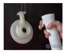
Figure 5. Spray isopropyl alcohol on the PolyCast™ SP802C pattern
