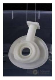
Figure 4. Dip the PolyCast™ SP802C pattern into isopropyl alcohol
